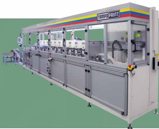
Reference Toy industry: Fully automatic 12-colour tampon printing system Performance: 24.000 printing parts/h
